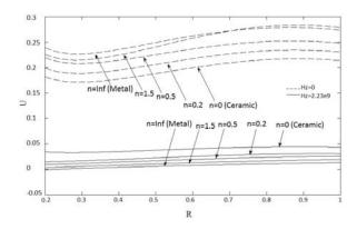
**Fig. 14**Comparing non-dimensional radial displacement with and without considering magnetic field for free-free boundary condition.
