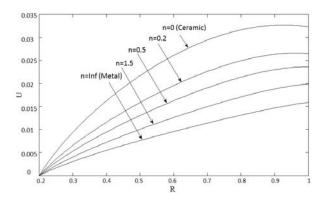
**Fig. 9**Distribution of non-dimensional radial displacement for fixed-free boundary condition.
