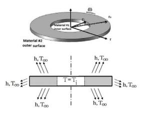
**Fig. 1** Configuration of a thin FG hollow rotating disk.
