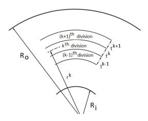
Fig. 2 Dividing radial domain into some finite sub-domains.
