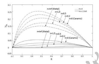
**Fig. 15**Comparing non-dimensional radial stress with and without considering magnetic field for free-free boundary condition.
