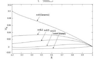
**Fig. 10**Distribution of non-dimensional radial stress for fixed-free boundary condition.
