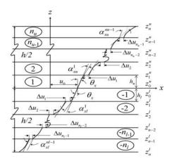
**Fig. 1** General lamination lay-up and displacement configuration.
