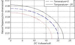
Variation of the fundamental frequency versus applied DC voltage for different temperature changes  $(T_r = 0, T_a = 0)$ .
