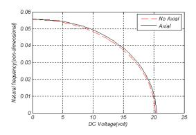
**Fig. 2** Variation of the fundamental frequency versus applied DC voltage with and without stretching  $(T_r = 0, \Delta T = 0)$ .
