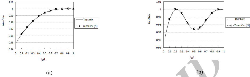
Fig. 2 Data validation for cracked FGM beam: non-dimensional natural frequency of cracked FGB versus non-dimensional crack location a) First natural frequency b) Second natural frequency.
