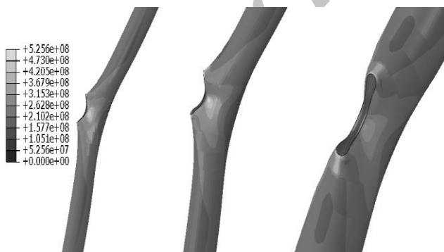
Fig. 19 Von mises stress contour for cylindrical shell under combined loading with 440mm length after 5 cycles.
