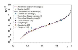
**Fig. 3** Comparison of the scale analysis model, Eq. (15), with the existing results in the literature (for  $\alpha$ =1).
