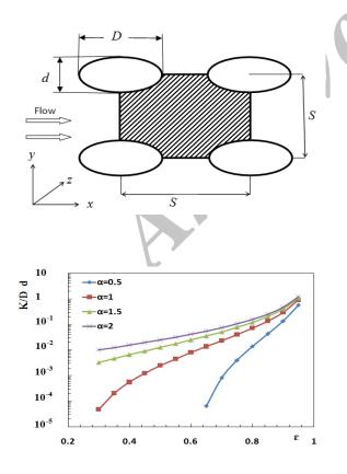
**Fig. 1** Unit cell for a composite with elliptical fibers.
