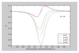
**Fig. 10**Variation of normal displacement w.r.t. horizontal distance in medium-II.
