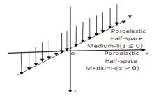
Fig. 2 A Normal line load of magnitude  $F_1$  per unit length acting along y-axis in the direction of +ve z-axis at the interface z = 0.
