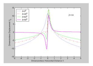
Fig. 5 Variation of normal displacement w.r.t. horizontal distance in medium-I.
