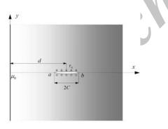
**Fig. 1** A crack embedded in a functionally graded semi-infinite plate.
