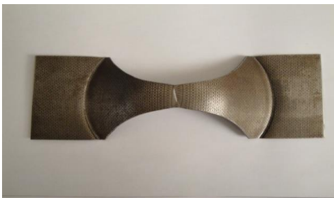
Fig.4 Sample stamped specimens used for FLD determination with fracture after testing.
