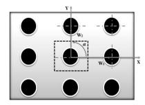
Fig.2 Schematic diagram of square fiber arrangements.
