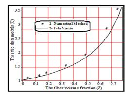
Fig.10 The variation of G versus different values of  $\xi$  for unidirectional glass fibers in a square pattern.
