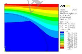
Fig.6 The distribution of temperature at temperature ( $T = 10^{-3}$ °C) on line y=1.
