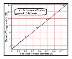
**Fig.8** The variation of  $E_1$  versus different values of  $\xi$  for unidirectional glass fibers in a square pattern.
