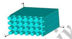
Fig.1 Schematic and coordinate of composite plate with unidirectional fibers.
