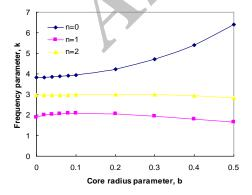
**Fig.2** Frequencies for small core radius parameter b, and v = 0.1 (G-G annular plate).
