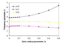
**Fig.6** Frequencies for small core radius parameter b, and  $\nu = 0.5$  (G-G annular plate).
