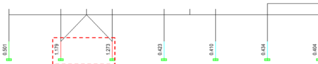
Figure 6. Critical condition of pedestals
