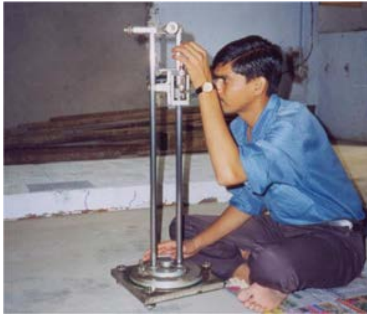
Figure 9 Microlevel deflection measurement equipment.
