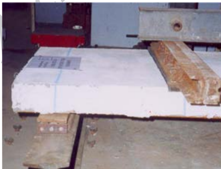
Figure 6 Actual view of roller support.
