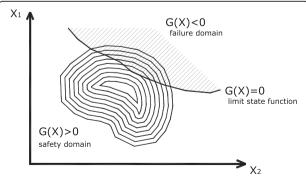
Figure 1 Domains of failure and safety for two random variables.
