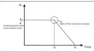
Figure 4 Corrosion process of the reinforcement cross-section area.
