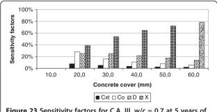
Figure 23 Sensitivity factors for C.A. III, w/c = 0.7 at 5 years of structural lifetime.
