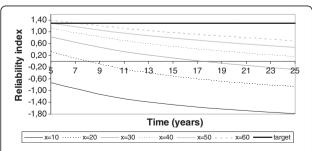
Figure 16 Abacus reliability index required for C.A. III and w/c ratio of 0.5.
