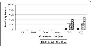
Figure 24 Sensitivity factors for C.A. III, w/c = 0.7 at 25 years of structural lifetime.
