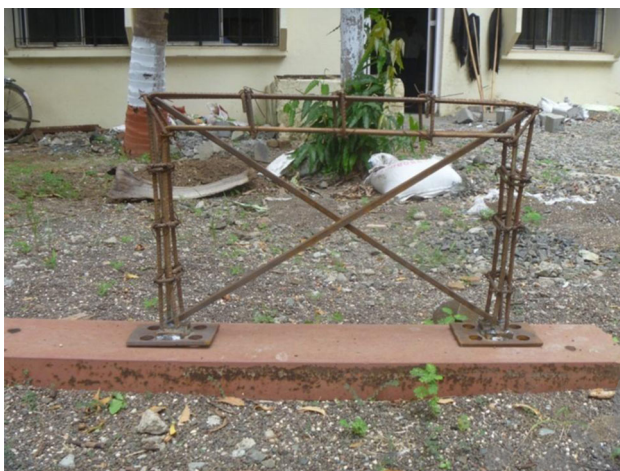
Fig. 2 Reinforcement details of frames
