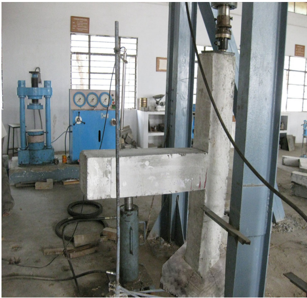
Fig. 7 Experimental test set-up of exterior beam-column joint
