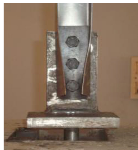
Fig. 12 Bending of the 2 mm thick packing plate with specimen
