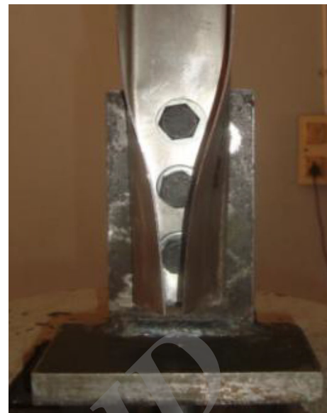
Fig. 10 Bending of unconnected leg of sample
