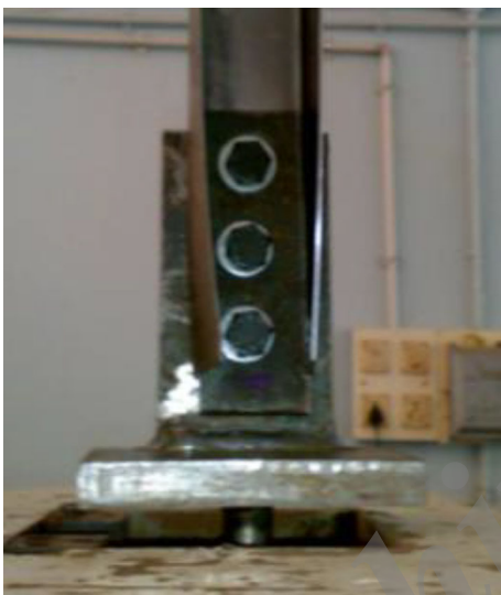
Fig. 36 Reduction bending of the 5 mm thick packing plate with specimen
