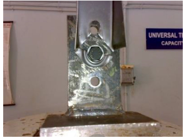
Fig. 43 Longitudinal shear failure observed for 1.5 mm thick specimen sample with single bolted connection
