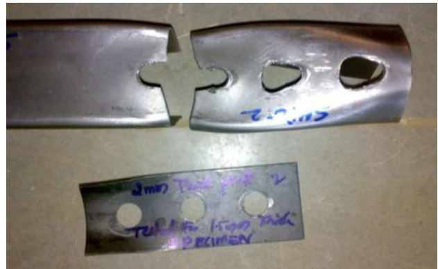
Fig. 38 Bearing + rupture failure observed with 2 mm thick packing plate for 1.2 and 1.5 mm thick specimen sample
