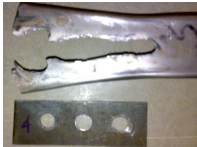
Fig. 40 Longitudinal shear failure of 1.5 mm thick sample specimen using 4 mm thick packing plate
