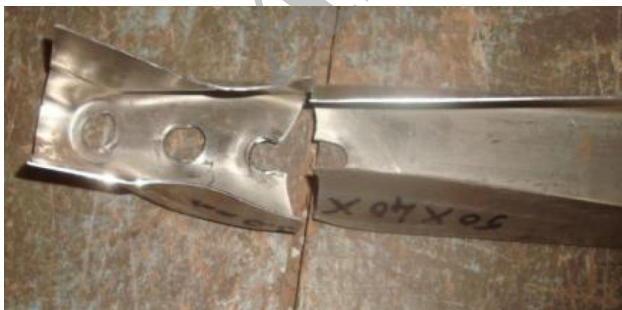
Fig. 37 Bearing + rupture failure observed
