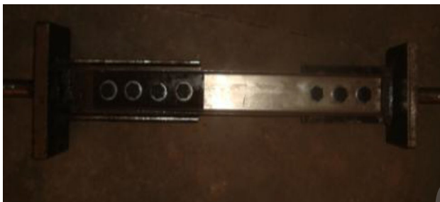
Fig. 7 Setup attached with CFS channel specimen
