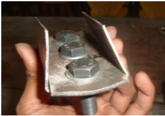
Fig. 35 Reduction bending of the 3 mm thick packing plate with specimen
