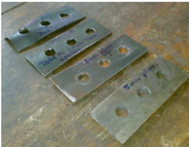
Fig. 42 Buckling of packing plate used 1.5 mm thick sample specimen
