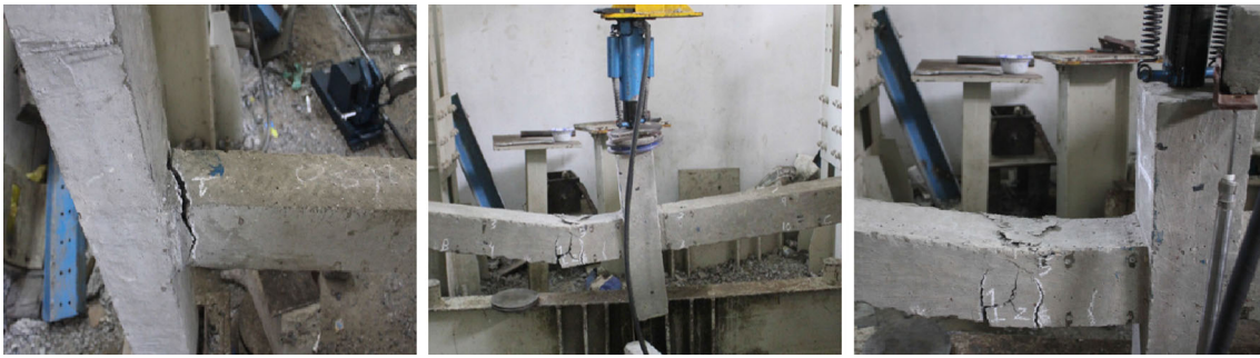
Fig. 11 Crack formation in specimen with monolithic connection (MC)
