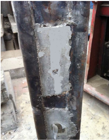
Fig. 4 Strengthened RC column specimen CS1 with steel angles and strips
