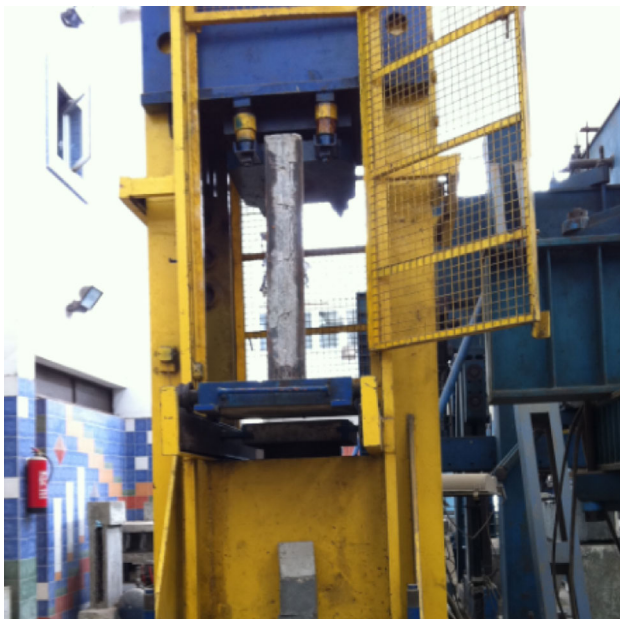
Fig. 5 Experimental testing machine of strengthened columns
