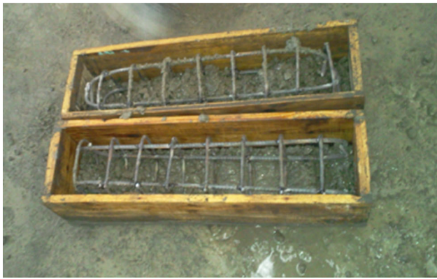
Fig. 1 Mesh reinforcement concrete beam and specimens
