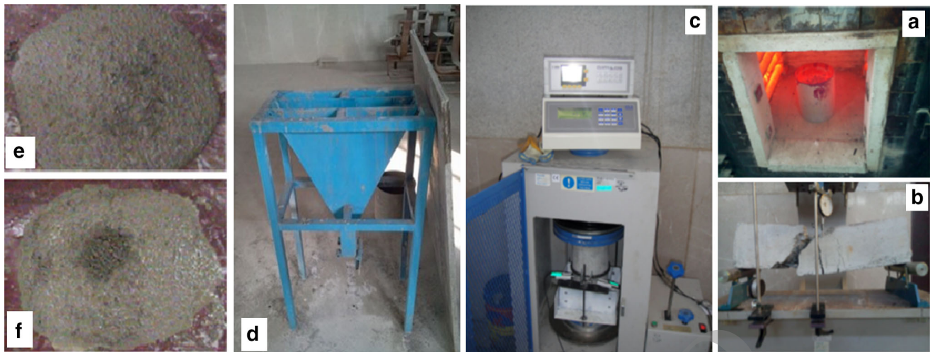
Fig. 2 Test machine (a heater, b bending test, c compressive test, d V funnel test, e, f slump flow test)
