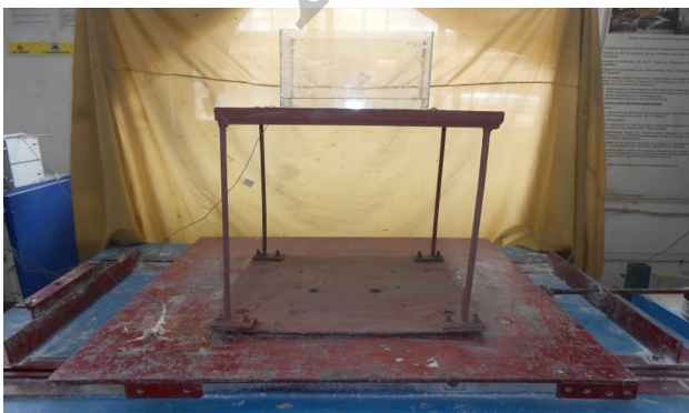
Fig. 1 Experimental setup of STLD-structure system
