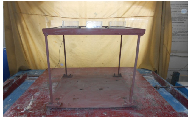
Fig. 2 Experimental setup of MTLT-structure system
