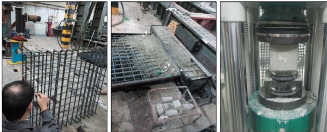
Fig. 3 Specimens' fabrication, concreting and compressive strength test
