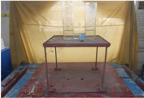
Fig. 1 LCVA-Structure Experimental setup
