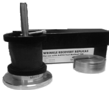
Figure2. Wrinkle recovery tester of Shirly corporation
