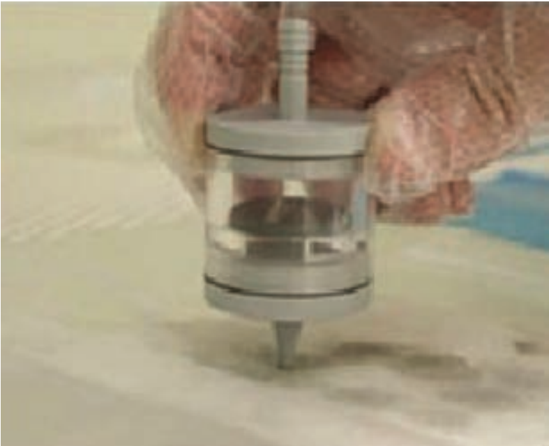
Figure 5: Collecting particulates from a surface using a suction pump
