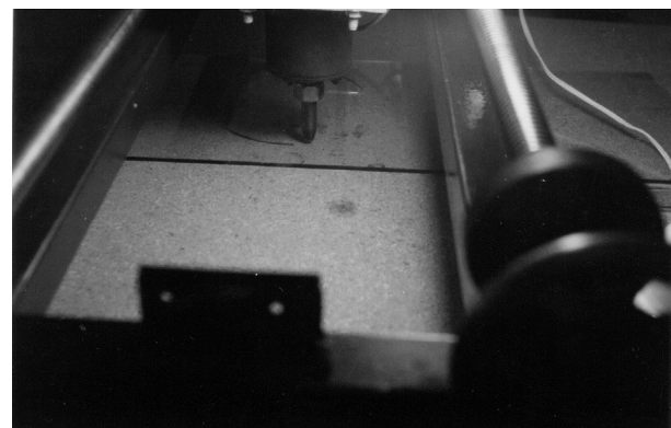
Fig. 2. Glazier on the instant of cutting a curve on a glass plate
