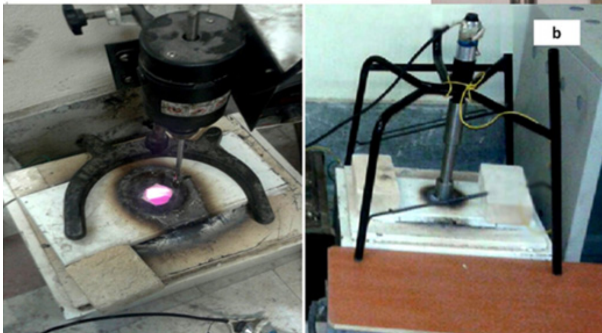
Fig. 4. a) Ultrasonic probe and (b) mechanical stirrer and ultrasonic device.
