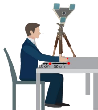
Fig. 1. A schematic of the experiment setup. The red dots indicate the three markers. The distance between each marker and the subject is shown.
