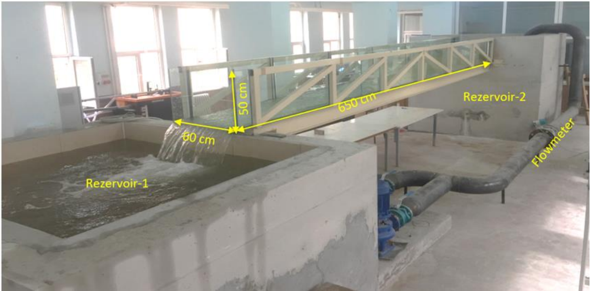
Fig 4: Open channel system used in experiments.
