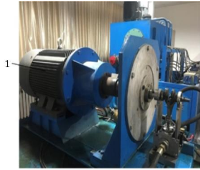
a) Hydraulic test-bed drive system
