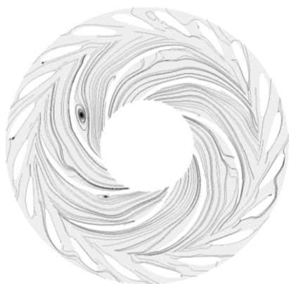
Fig. 11. Flow inside the impeller Q/Q_{opt} = 0,73 – hump zone.
