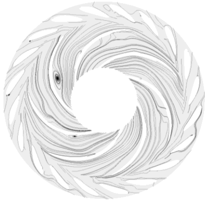
Fig. 11. Flow inside the impeller Q/Q_{opt} = 0,73 – hump zone.
