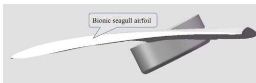
Fig. 2. Designed bionic seagull airfoil profile.
