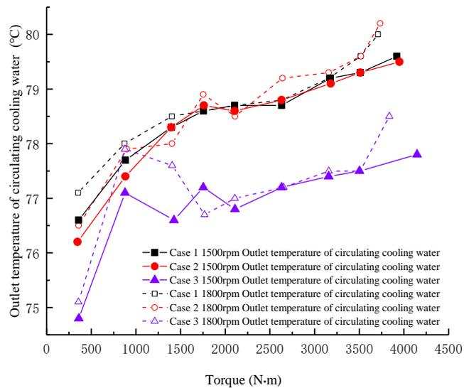
Fig. 7. Outlet temperature of the circulating cooling water at different engine speeds.
