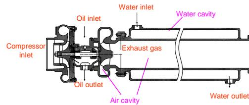
Case 2 Water cooling exhaust pipe and air-cooling turbine case
