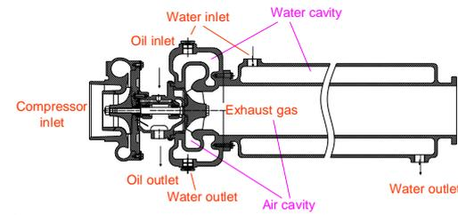
Case 1 Water cooling exhaust pipe and water-cooling turbine case
