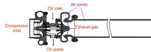
Case 3 Air cooling exhaust pipe and air-cooling turbine case
