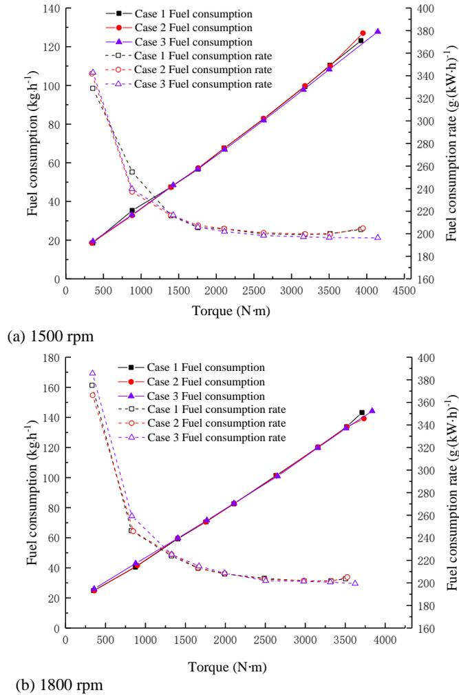
**Fig. 5. Fuel consumption at different engine speeds.**
