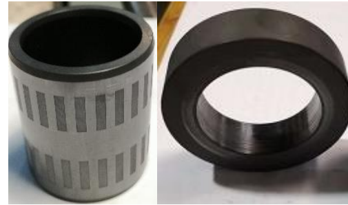
(a) rotary ring (b) stationary ring Fig. 6. Specimens of rotary and stationary rings.
