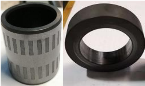
(a) rotary ring (b) stationary ring Fig. 6. Specimens of rotary and stationary rings.
