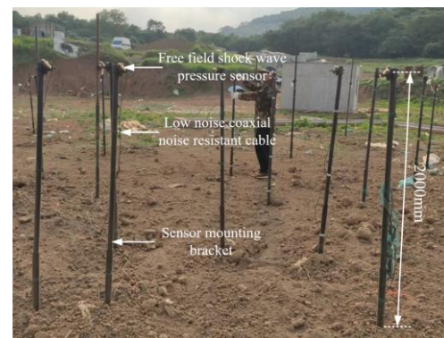
Fig. 9. Field layout of the free-field shock wave pressure sensor.
