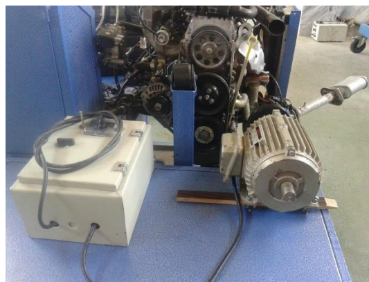
Figure 1: Motor setup, electric motor and inverter
