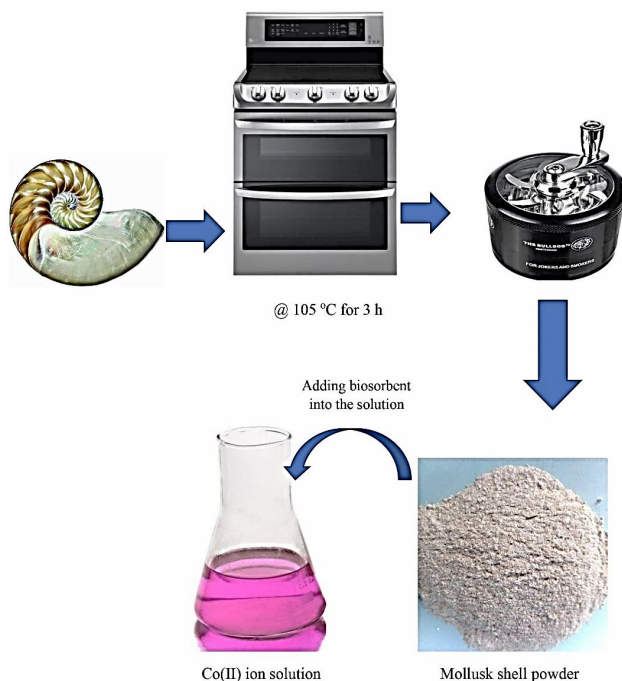
Fig. 1. Schematic of the biosorbent production and its use in eliminating \text{Co}^{2+} ions from aqueous solution.
