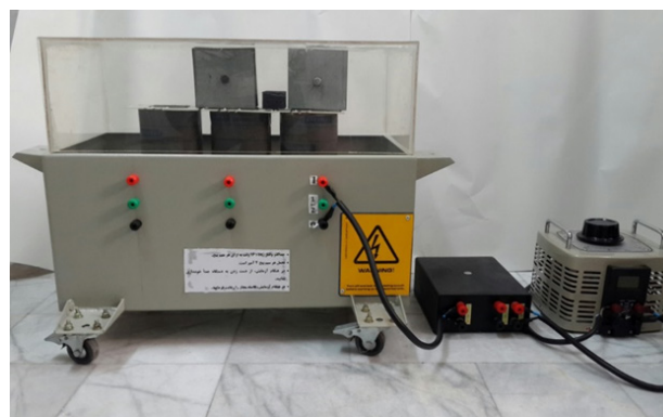
Fig. 1. Magnetic field generator, rectifier and a VARIAC Variable Transformer used in current study to apply static magnetic field on Fibroblast cells.
