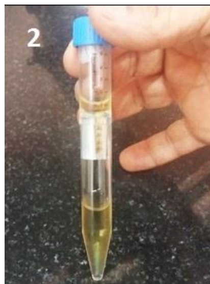
Figure 2: Concentrated ECP of Y. ruckeri using centrifuge protein purification. Upper phase in filter refers to concentrated ECP.
