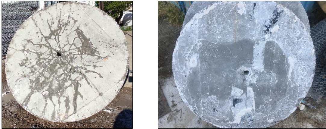
Figure 15. Concrete Slab under the uniform loading: (a) with rigid anchorage system; (b) with deformable anchorage system.
