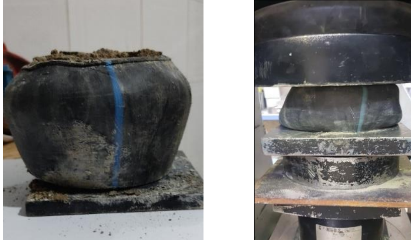
Figure 6. Deformability capacity of HDC element under compressive pressure.
