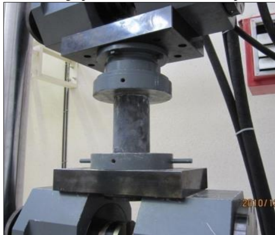
Figure 5. UTM loading machine.
