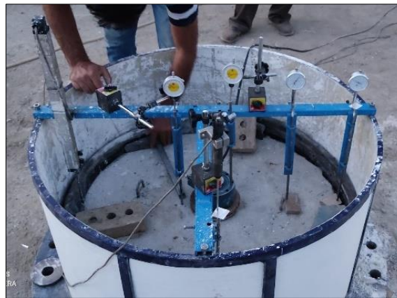
Figure 11. The concrete slab test setup.
