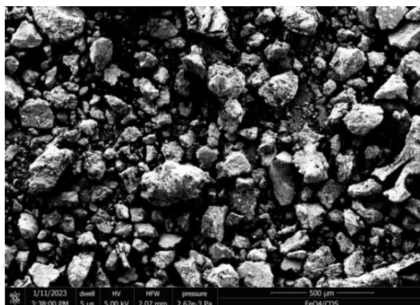
Fig. 3. The SEM photograph of \text{Fe}_3\text{O}_4/\text{CDs} nanocomposite.
