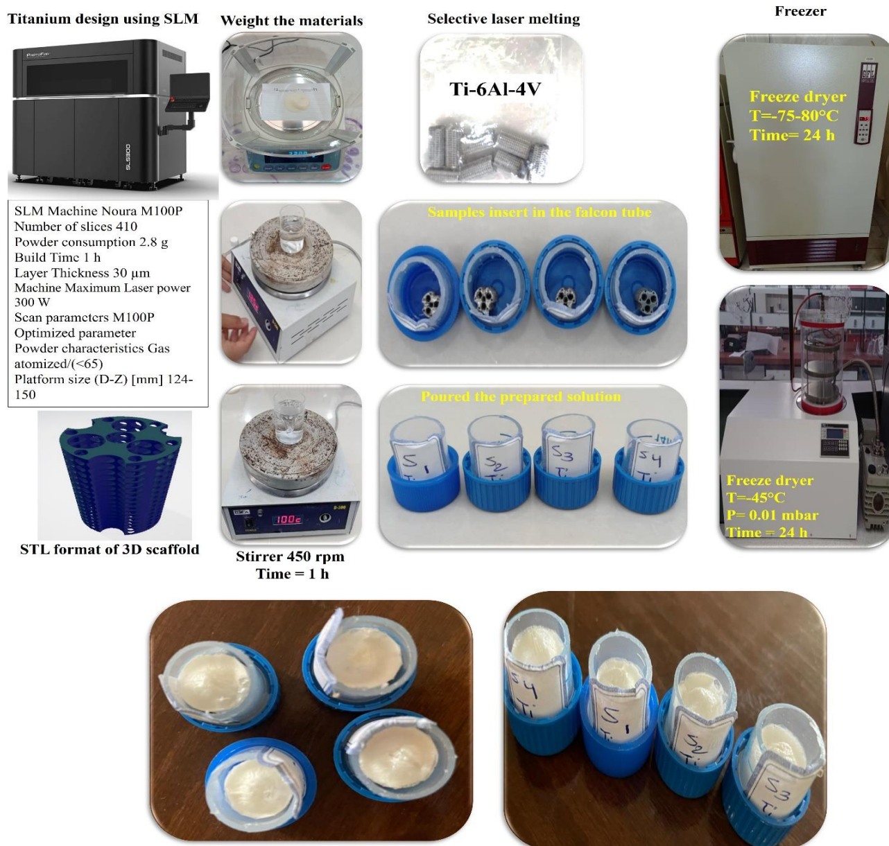
Fig. 4: Sample preparation steps with freeze drying polymer coating with wollastonite nanoparticles
