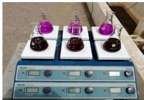
Fig. 1: Experimental set up used for solar degradation of DV 51.
