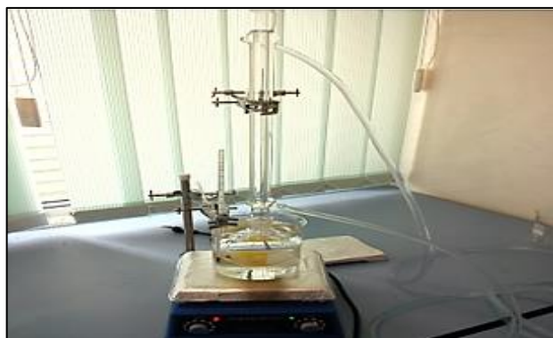
Fig. 2: Esterification using reflux and water bath method.
