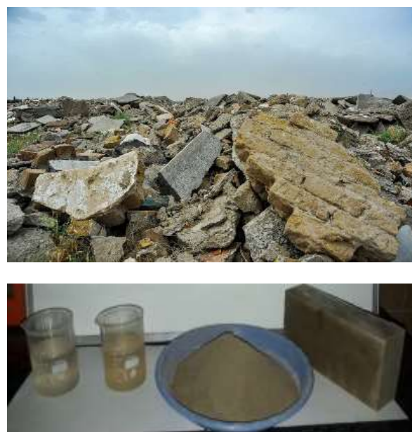
Fig. 1. Demolishing waste containing CBW (Top), and CBW powder, alkaline solutions and CBW-based geopolymeric brick (Bot)
