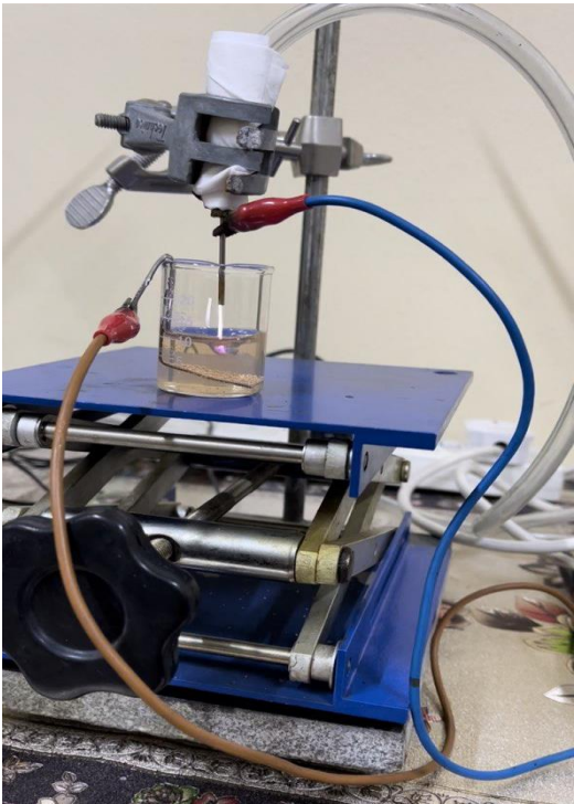
FIGURE 1 The cold plasma system using to prepare SeNPs
