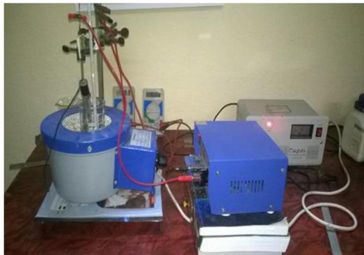
Figure 1 (b). Galvanostatic linear electrodeposition setup.
