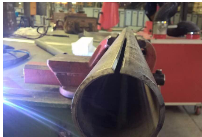
Figure 2. The sample type with a 60 degree chamfer
