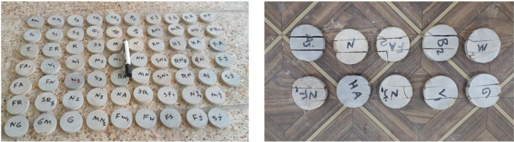
Figure 4. Some of specimens before and after failure in the BPI test
