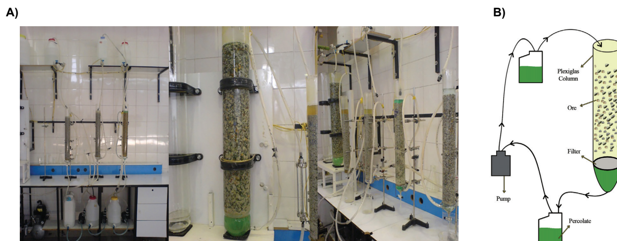
Figure 1. Percolation column. A) Real setup. B) Schematic diagram.
